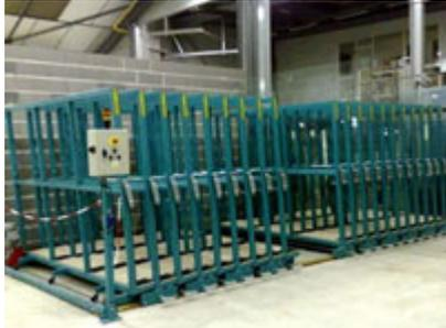
The mobile frame racks is a solution for storing metal sheets in a vertical manner. This space saving storage system consists of a number of drawers that are provided with wheels to make them easy to shift. Moving a pack of drawers to the left or the right creates an aisle that provides the necessary space to easily load or unload the metals sheets from the drawer. Eurostorage delivers this type of storage in a manual and an electric version.
