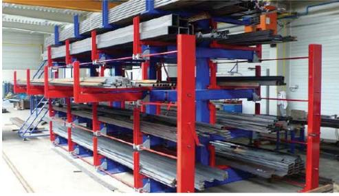
The roll cantilever rack is a compact and secure storage system for tubes, pipes, bars, ... The levels are for 100% extensible outside the rack. This type of rack is available in a manual and automated version. Besides that type of storage of profiles, Eurostorage also delivers the cantilever with pivoting arms.
