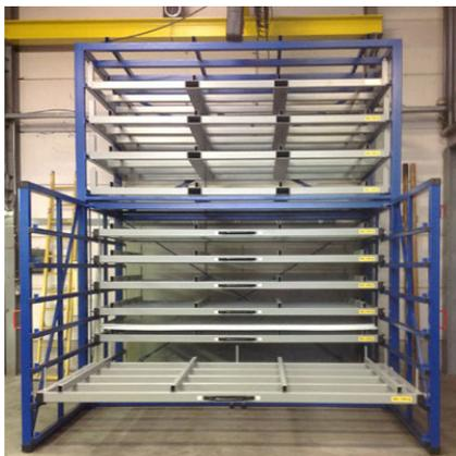
The metal sheet warehouse rack is a compact system on a small floor space. The block on the floor consists of drawers that can be pulled out for 100% and the block above contains cassettes for use with a forklift.
