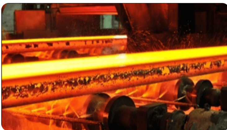
Fig 1: Hot slabs immediately after casting
