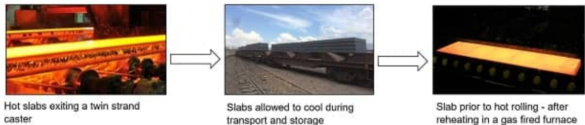
Fig 3: Most hot mills making automotive products reheat slabs that have cooled during transport and storage.
